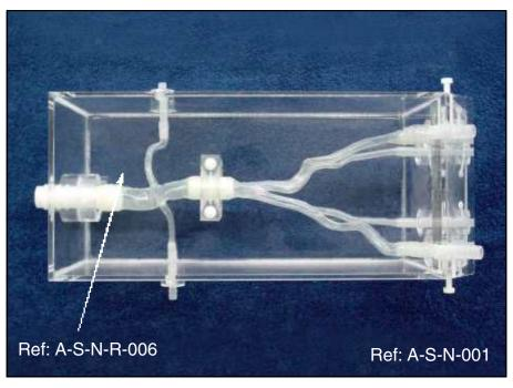
Abdominal aorta model including the renal arteries and the bifurcation of the common iliac arteries. This model can be used to teach renal artery catheterization technique. It allows realistic testing of endovascular devices and PTRA therapy.
