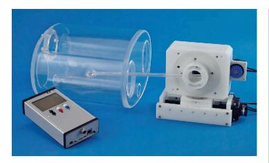
Shelley Medical's programmable multi-modality Respiratory Tumour Motion Phantom simulates accurate and reproducible tumour motion from patient-specific breathing profiles. The Respiratory Tumour Motion Phantom is ideal for commissioning of new systems and system upgrades/repairs, scheduled testing, quality assurance tests and comparative testing of PET, MRI & CT in radiotherapy planning where respiratory motion is of concern.
